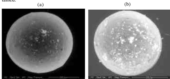
**Figure 3: SEM of Batch MS4 (a) before and (b) after *in vitro* drug dissolution**
