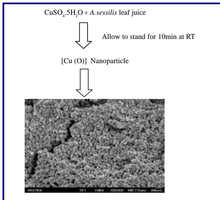
Fig 1: Schematic formation of Cu (O) nanoparticles by reduction method
