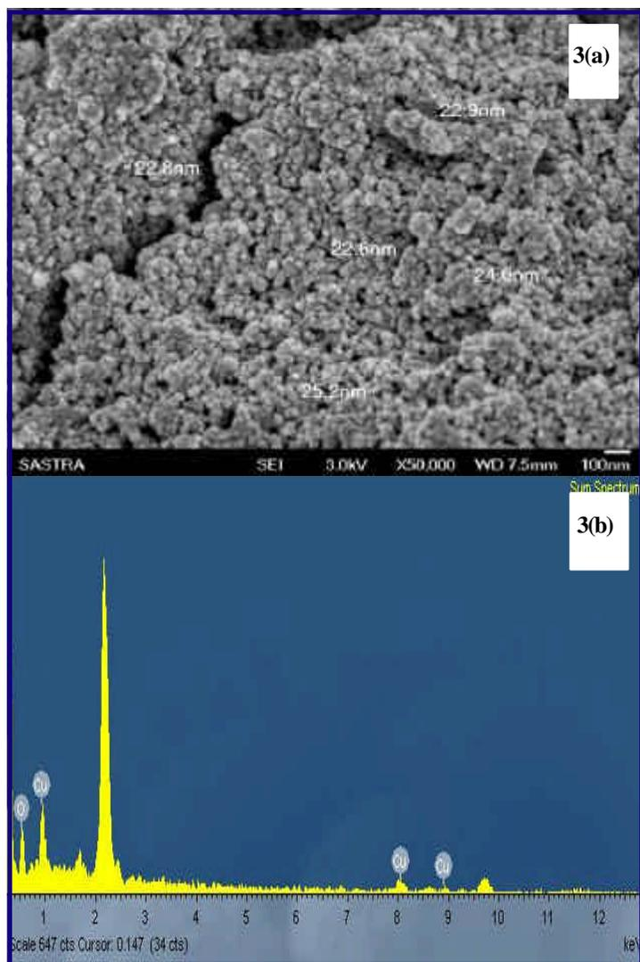
Fig 3(a, b): SEM images and EDAX spectrum of CuO nanoparticles
