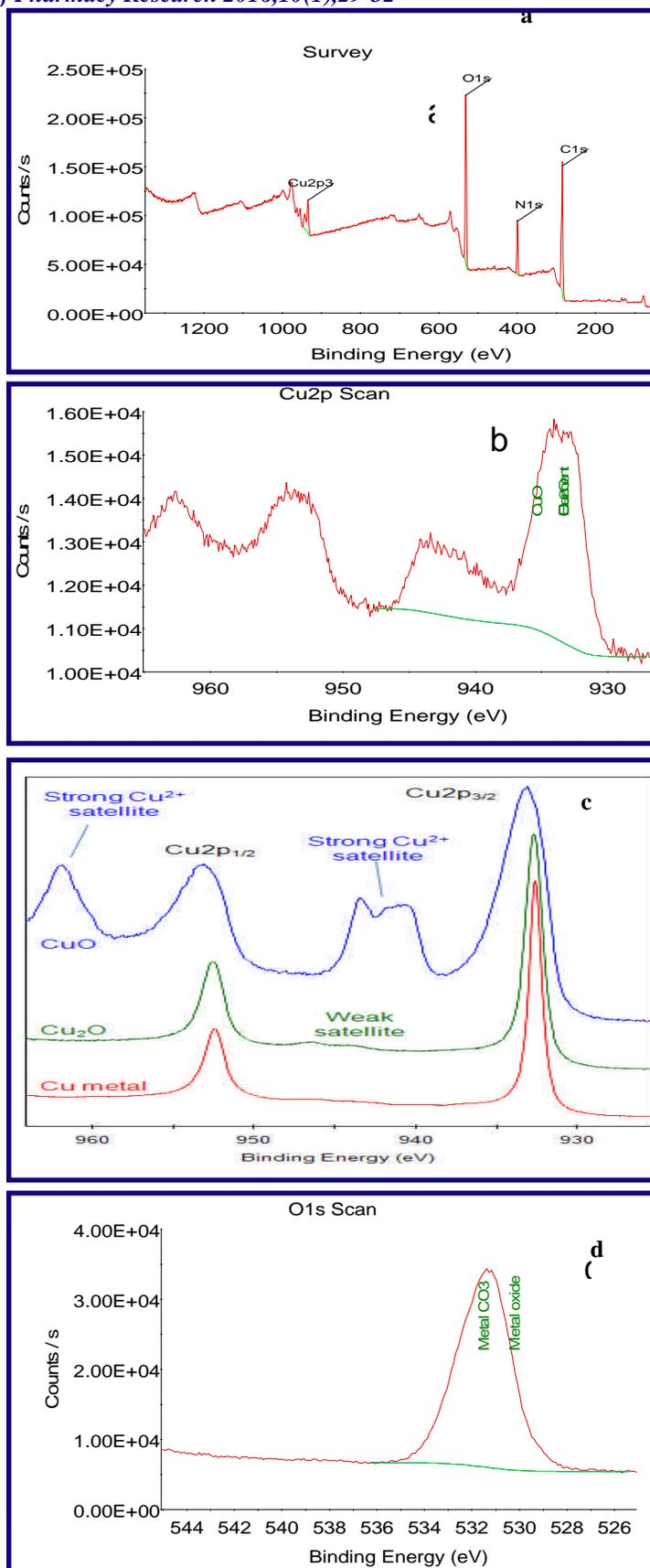
Figure 4: XPS spectra of (a) survey scan (b) Cu2p scan (c) core level spectrum of Cu2p<sub>3/2</sub> (d) O1s scan
