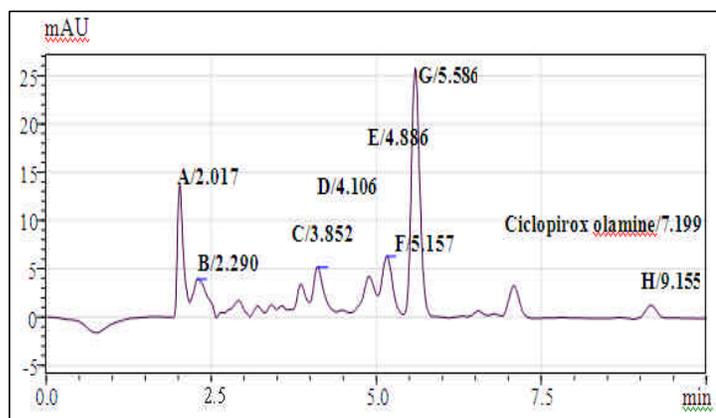
Degradation products found and separated after sunlight degradation are shown as alphabet A-H with their retention time. Observed peak of degradation products are well separated from the peak of drug
