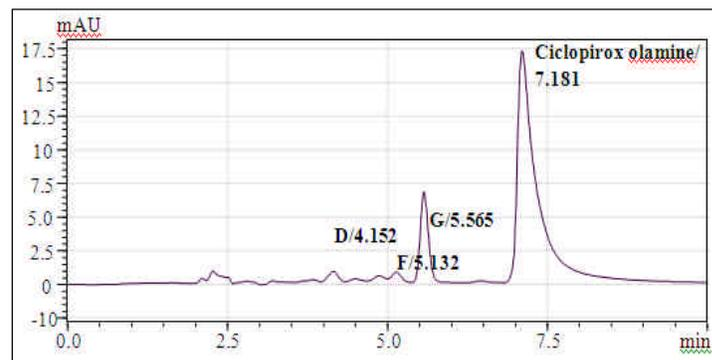
Degradation products found and separated after UV light degradation are shown as alphabet A-H with their retention time. Observed peak of degradation products are well separated from the peak of drug
