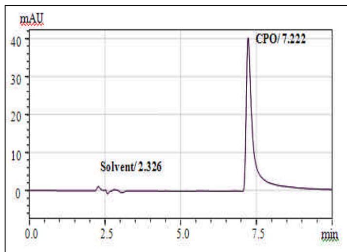
Ciclopirox olamine (CPO) with corresponding retention time (tR) of 7.222 min was detected at 305 nm. Peak of solvent observed at tR of 2.326 min is well separated from peak of drug
