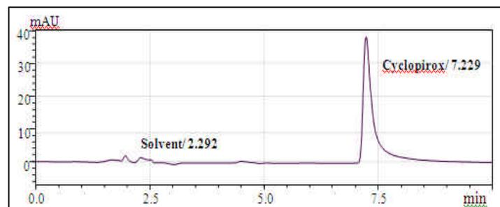
**Figure 4: Purity plot of CPO at 305 nm by stability indicating RP-HPLC method**
