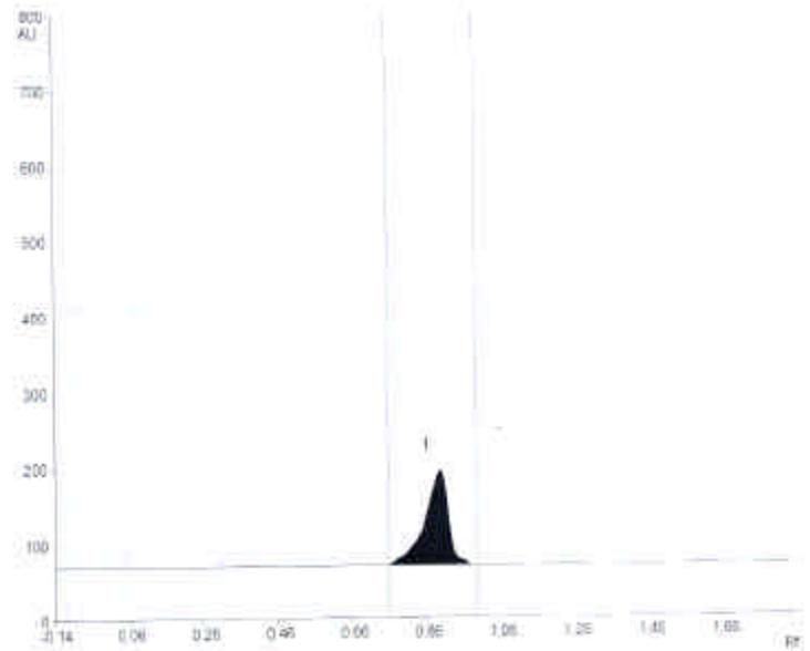
**Figure 2 HPTLC Chromatogram of Isovannillin in Raw material**
