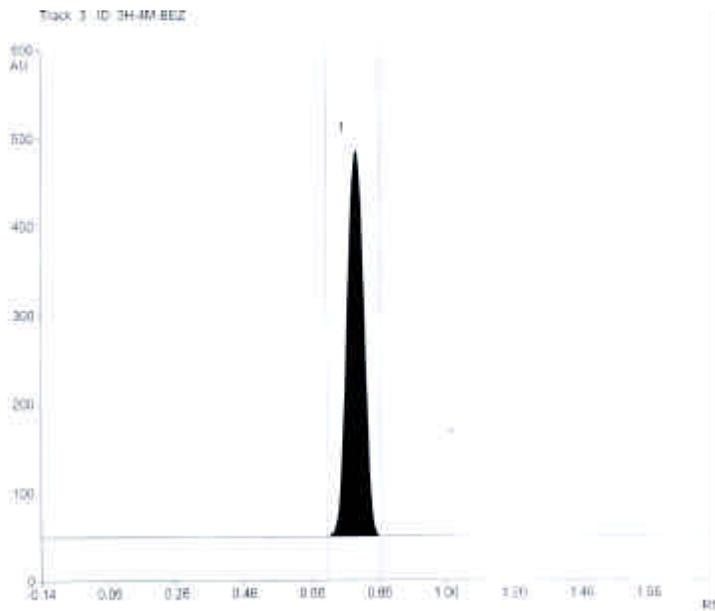
**Figure 1. HPTLC Chromatogram of standard Isovannillin**
