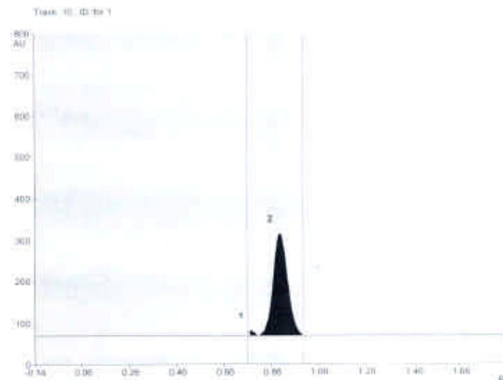
**Figure 5. HPTLC Chromatogram of Isovanillin in Formulation**
