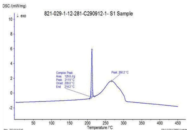
Figure 6: DSC thermogram of Venlafaxine HCl
