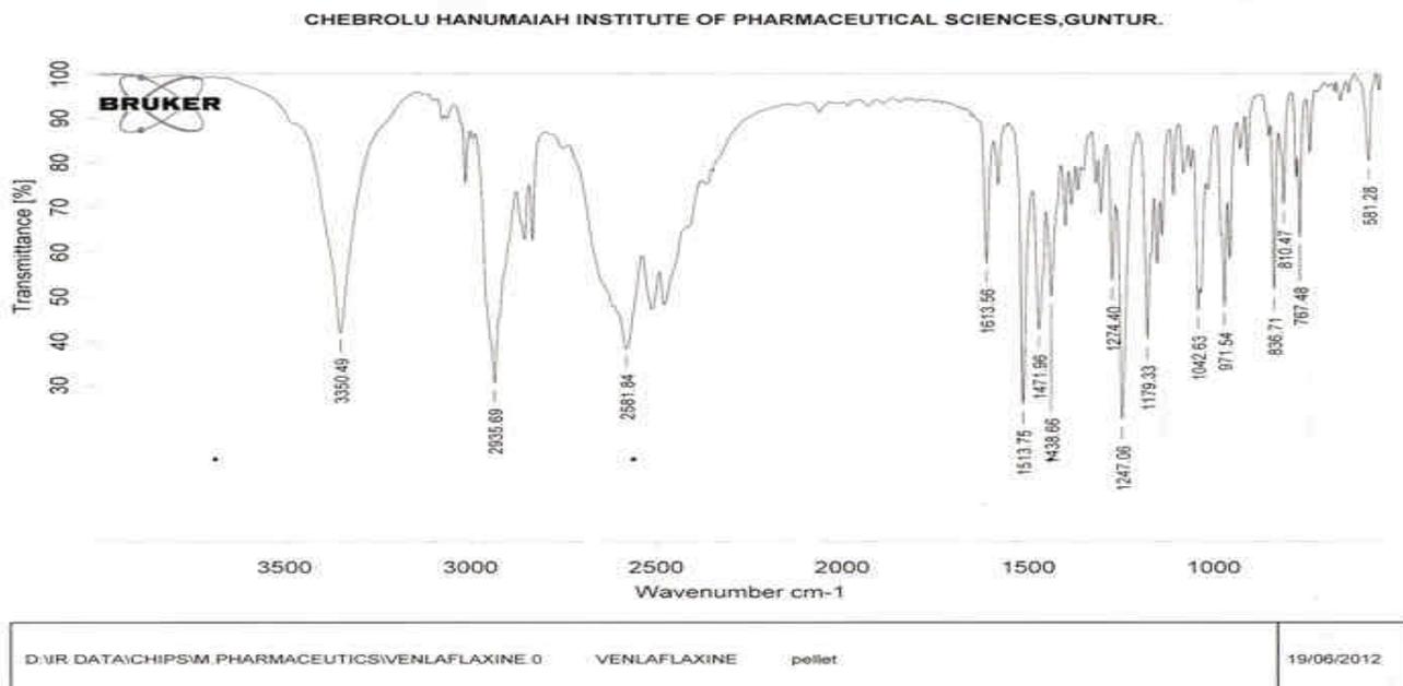
Figure 3: FTIR spectra of Formulation Venlafaxine HCl
