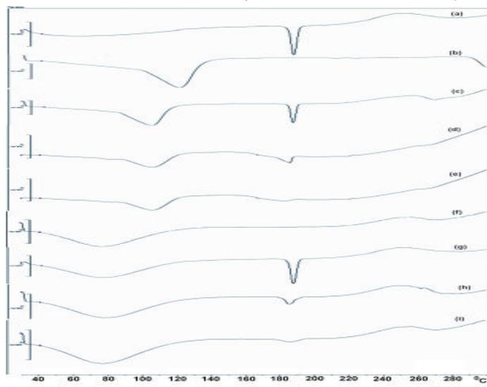
Fig 5: DSC thermograms of Irbesartan, CD's and its complexes (a) IRB, (b)  $\beta$ -CD, (c) PMB, (d) COB, (e)KNB, (f) HP  $\beta$ -CD, (g) PMH, (h) COH, (i) KNH
