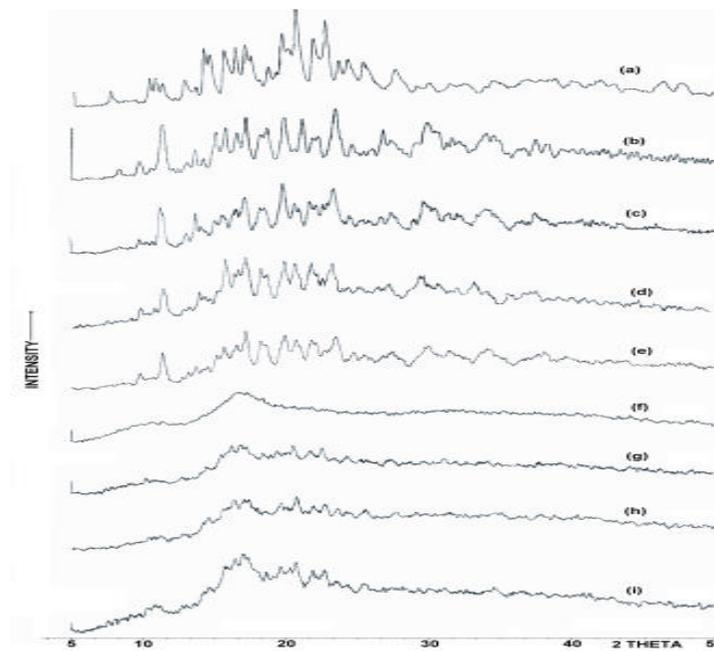
**Fig 4: PXRD Spectra of Irbesartan, CD's and its complexes (a) IRB, (b)  $\beta$ -CD, (c) PMB, (d) COB, (e)KNB, (f) HP  $\beta$ -CD, (g) PMH, (h) COH, (i) KNH**
