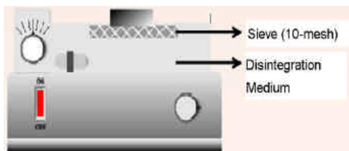
**Figure 1: Device Used to Determine the Disintegration Time of Fast Disintegrating Tablets**
