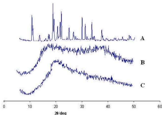
**Figure 3: X-ray diffraction patterns of Zolpidem tartrate (A), Tulsion 335 (B) and Resinate(C)**
