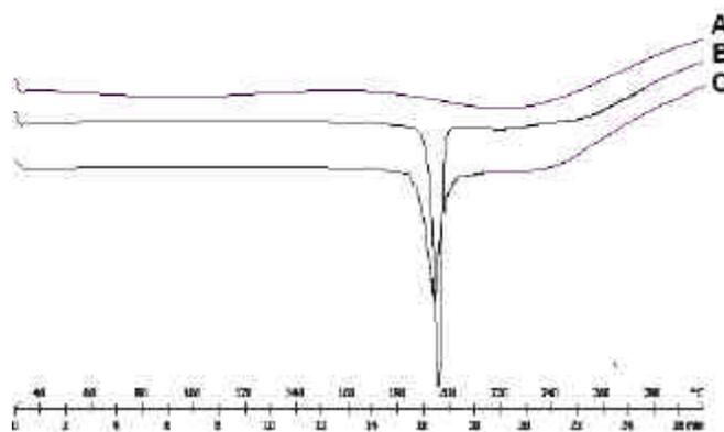
**Figure 2: DSC Thermograms of Tulsion335 (A), Zolpidem Tartrate (B) and Resinate(C)**
