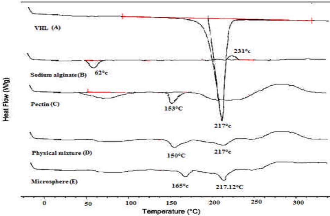
Figure3. DSC thermo grams of VHL, sodium alginate, pectin, physical mixture and microsphere
