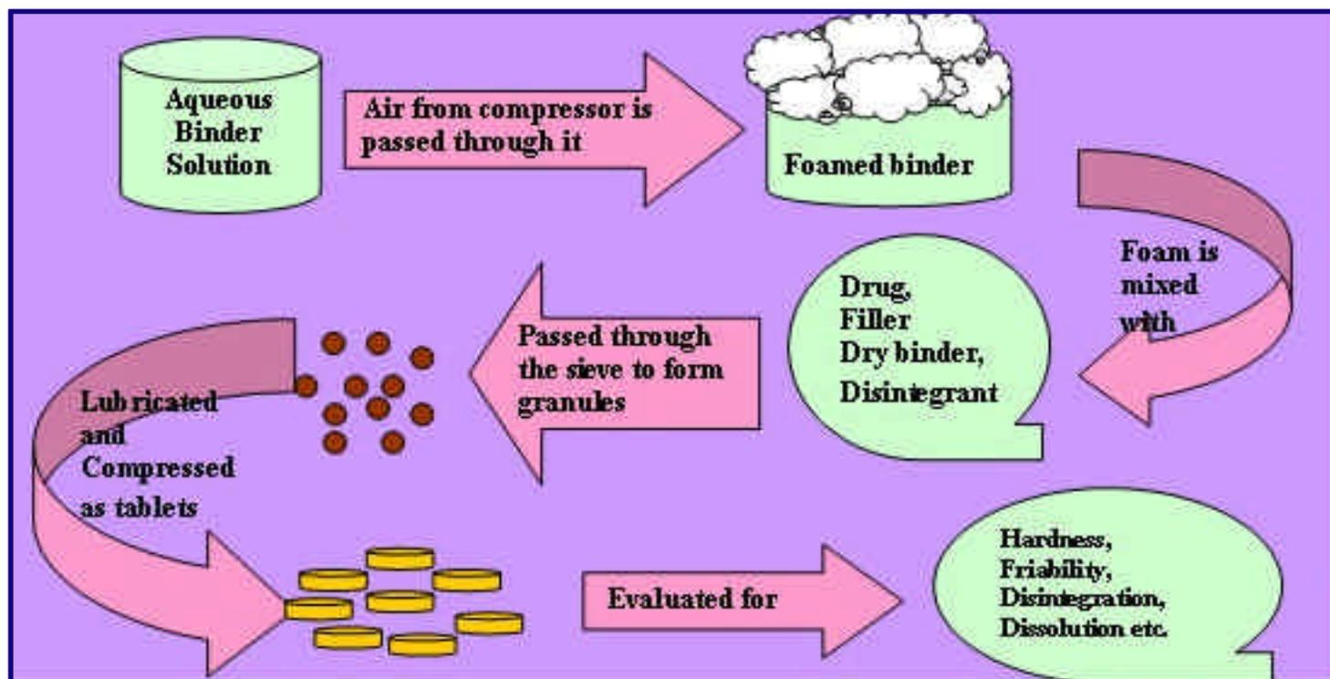
Figure 1. Schematic representation of foam granulation technology.
