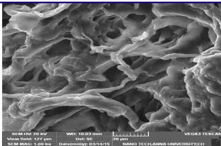
**Fig. 3b : SEM image of TLE incorporated Collagen**
