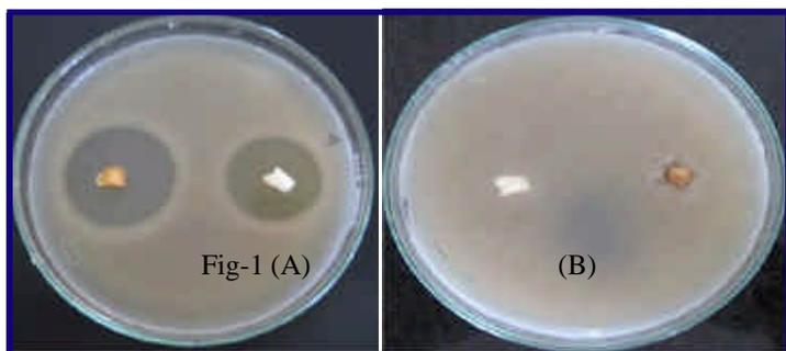
Fig-1(A) Zone of inhibition against *E. coli* (ATCC 43894) and *S. aureus* (ATCC 29213) exhibited by synergistic drug treated cotton. (B) Zone of inhibition against *E. coli* (ATCC 43894) and *S. aureus* (ATCC 29213) exhibited by untreated cotton
