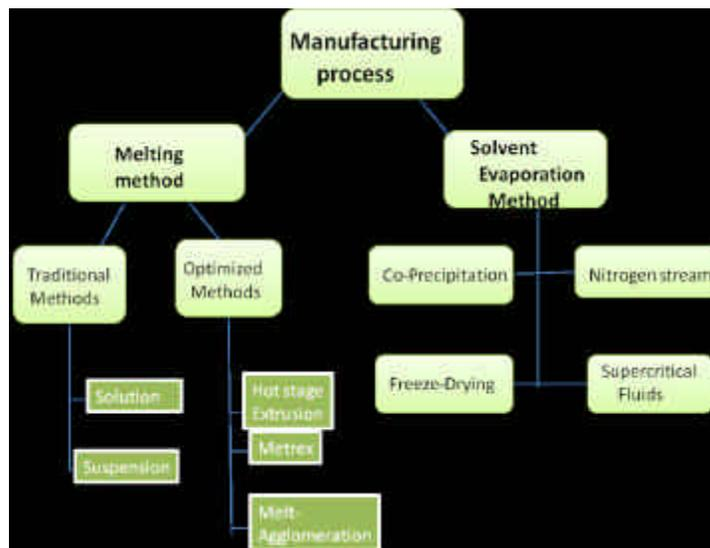
**Fig 2: Diagramatic representation is shown as below:**
