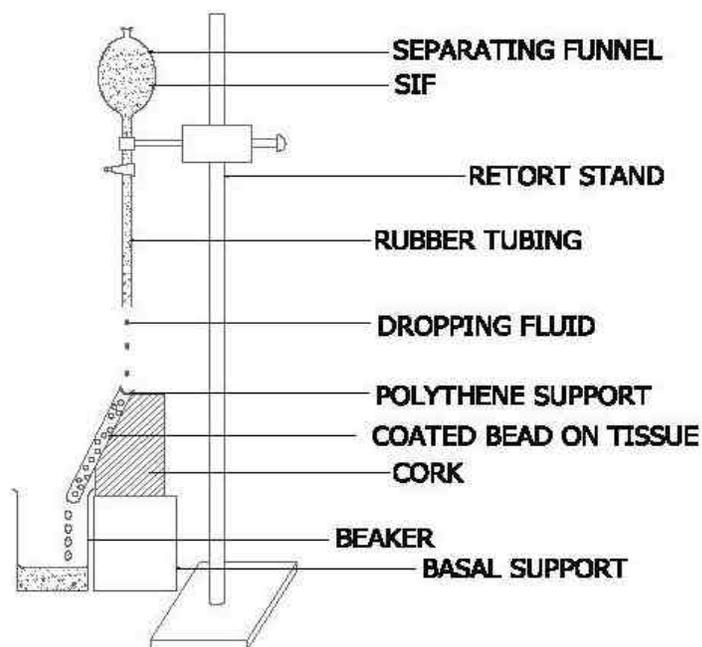
**Figure 1: Apparatus for bioadhesion of coated beads**
