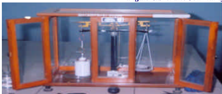
Figure 2. In-vitro mucoadhesive strength measurement apparatus
