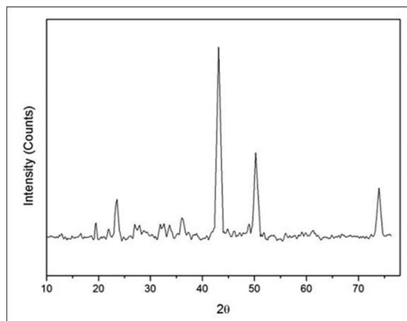
**Figure 2:** X-ray diffraction pattern of copper powder
