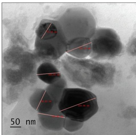
**Figure 6:** Represents transmission electron microscopy analysis of copper powder
