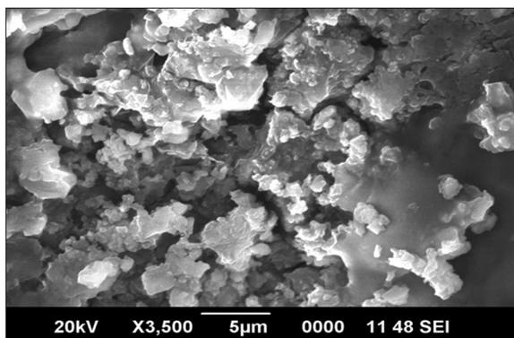
**Figure 5:** Scanning electron microscopy analysis of copper powder
