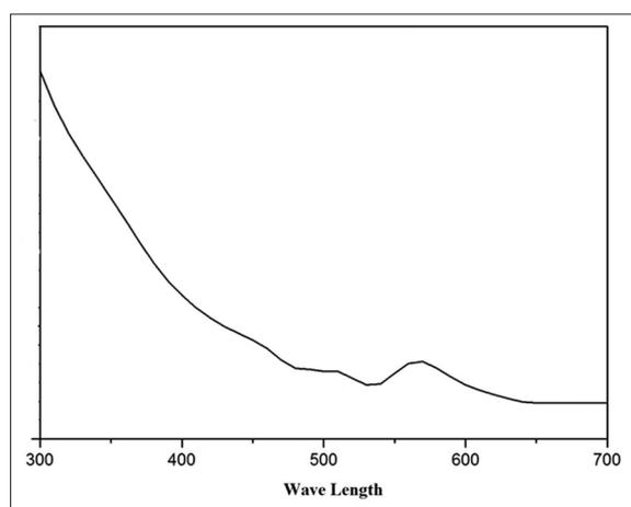
**Figure 3:** The ultraviolet-visible spectra of copper powder
