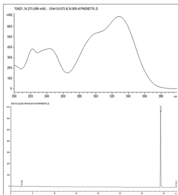
**Figure 1: Chromatogram and ultraviolet profile of a standard sample of caffeic acid phenethyl ester**
