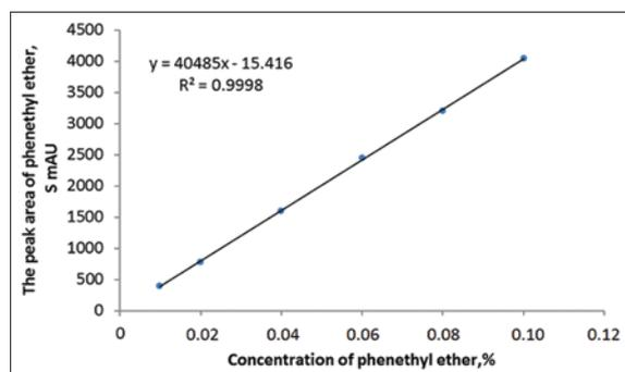
**Figure 5:** Calibration plot of the peak area of caffeic acid phenethyl ester against the concentration
