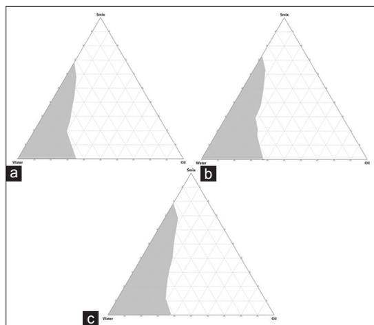
**Figure 3:** Pseudoternary phase diagram of system with the following components: oil = Capmul MCM, surfactant = tween 80, and cosurfactant = polyethylene glycol 400. Smix ratio of a is 1:1, b is 2:1, and c is 3:1
