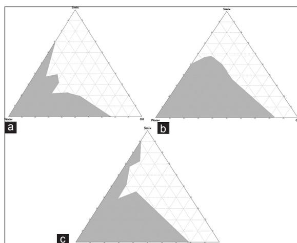
**Figure 2:** Pseudoternary phase diagram of system with the following components: Oil = Oleic acid, surfactant = Tween 80, and cosurfactant = polyethylene glycol 400. Smix ratio of a is 1:1, b is 2:1, and c is 3:1
