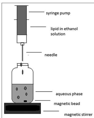
**Figure 1:** Schematic representation of assembly used in nanoliposome preparation
