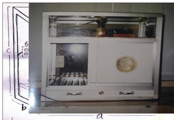
**Figure 1:** Humidity cabinet. a (length 60 cm); b (width 40 cm); c (height 59.5 cm); c1 (height 50 cm); c2 (drawer height 9.5 cm); 1 (roof of humidity cabinets); 2 (drawer where silica gel placed); 3 (handholes equipped with rubber gloves); 4 (lamp); 5 (hygrometer and thermometer); 6 (electric socket); and 7 (aluminum bars)
