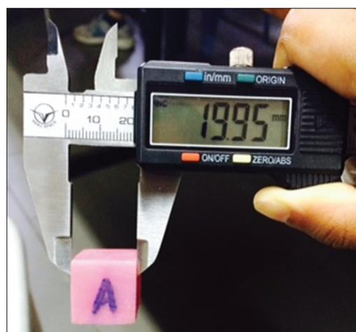
**Figure 2:** Measurement using digital vernier caliper
