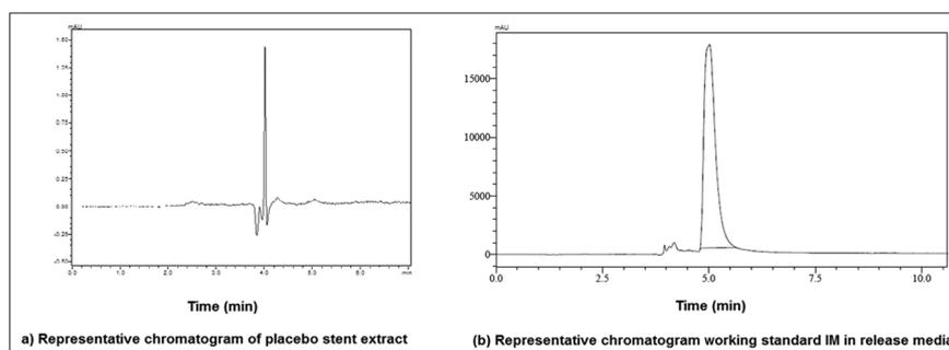
**Figure 3:** Representative chromatogram of placebo stent extract and working standard imatinib mesylate in release media
