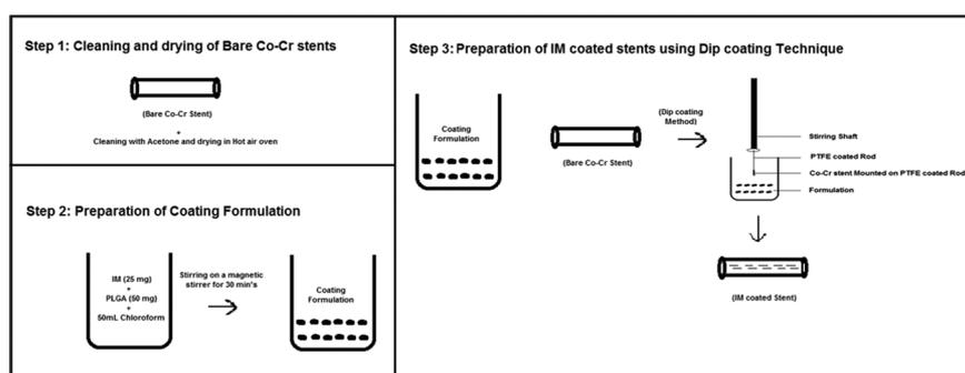
Figure 2: Schematic representation of dip-coating method
