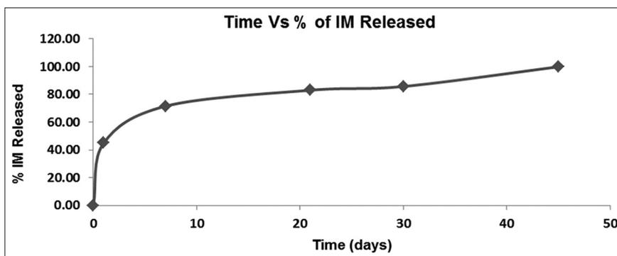
**Figure 4:** Release kinetics of imatinib mesylate (IM) from IM-coated stents
