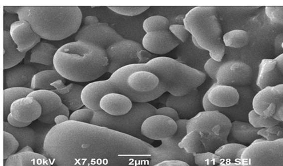
Figure 6: SEM image at 2 micrometer of 20% M.D Sugarcane juice powder at 170°C
