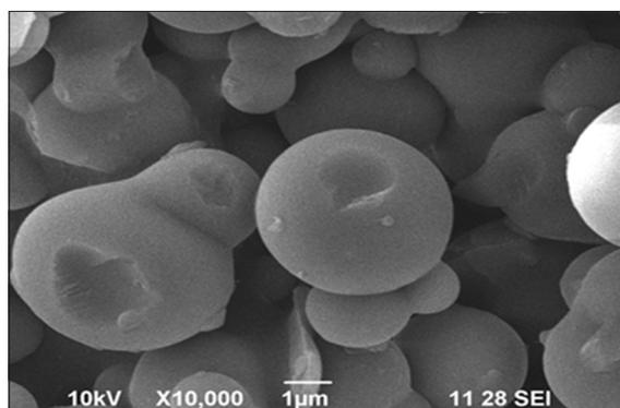
Figure 5: SEM image at 1 micrometer of 20% M.D Sugarcane juice powder at 170°C
