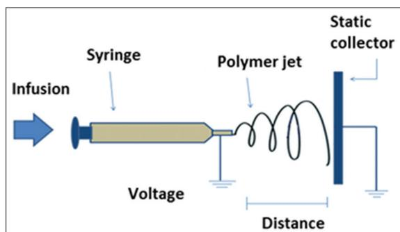
**Figure 2:** Typical electrospinning set up. Adapted and reconstructed from Pham *et al.*<sup>[28]</sup>
