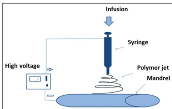
**Figure 3:** Schematic figure of electrospinning set up with rolling collector (mandrel)
